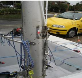
One rusty spanner, fits the bottle screw perfectly and the snapshackle stops it unwinding accidentally, you can easily adjust this between races.
