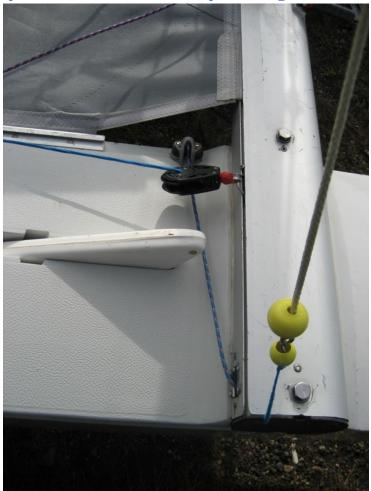
The ratchet block has a small self tapping screw into the beam to its port side. This prevents the block sliding over to the trampoline and getting caught up. It also leaves the rotation cleat fixed to the deck, clear to operate cleanly.
